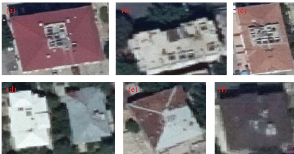
Figure 3. Different roof types: a) burgundy painted trapezoidal sheet, b) flat building, c) tile covered roof, d) sinus corrugated sheet, e) rusted sheet roof and f) shingle roof.
